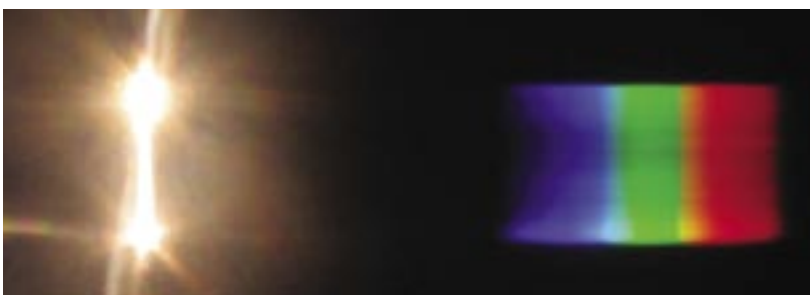
Figure 1c: Light from a regular incandescent light bulb, viewed through a spectroscopy. The range of colors is a smooth continuum.
